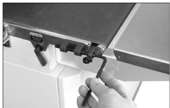
Figure 8-3: belt tension adjustment
