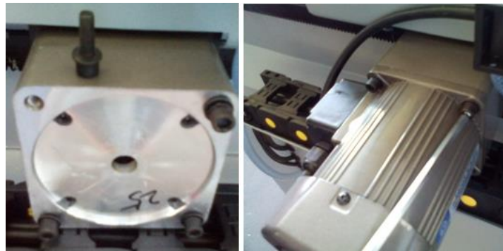
2. Travelmotor Mount with 4 screws
