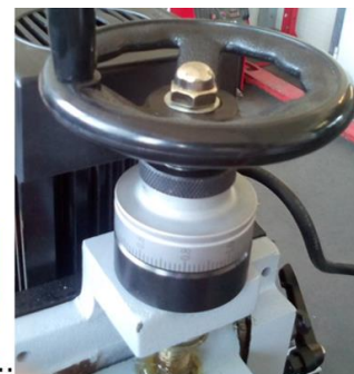
5. Handwheel: Place the handwheel and fix with the nut.
